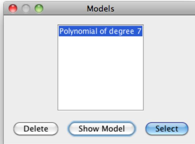
A model can be deleted via the `Delete` button. The `Select` button is used to select the highlighted model in the list for viewing on the Plot Pane and the Model and Residuals lists.
