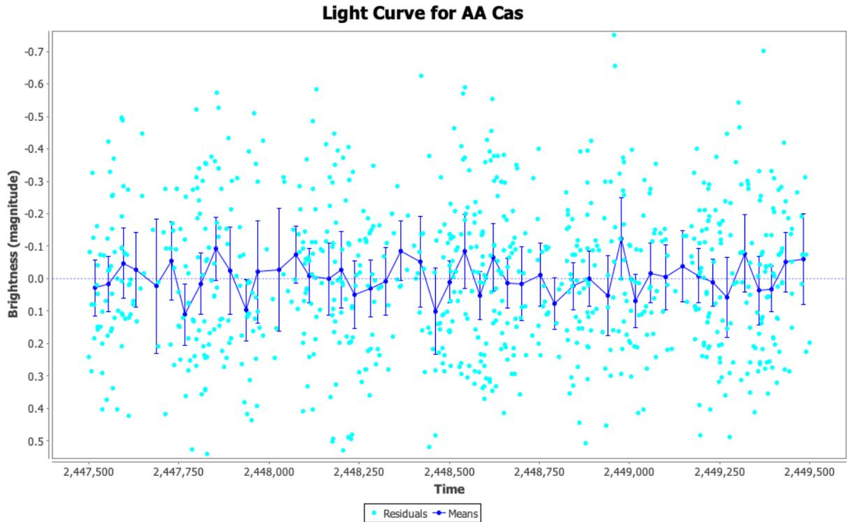
The Current Mode ANOVA plug-in could be used to show that what is observed in the residuals is likely to be due to noise rather than due to the presence of a non-trivial signal.
