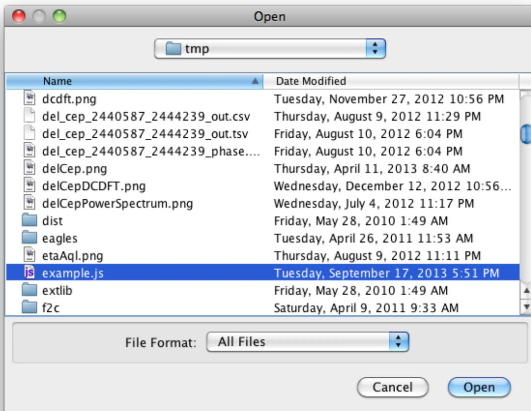
The file chooser shows `example.js` being selected. Clicking the `Open` button will cause the script to be executed. The example script will load data for eta Aquilae in the JD range 2455821.5...2456552.5, create a phase plot, and save it as a PNG file. It will repeat this for beta Lyrae.
